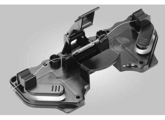
3M<sup>™</sup> Fibrlok<sup>™</sup> optical splice is a leading mechanical splice and is specified in fiber-to-thepremises projects as a substitute for fusion splicing. It provides a precise, simple and low-cost method of splicing optical fibers without electrical power. The Fibrlok splicing system is designed to minimize the need for lengthy training, specialized skills or experience.
